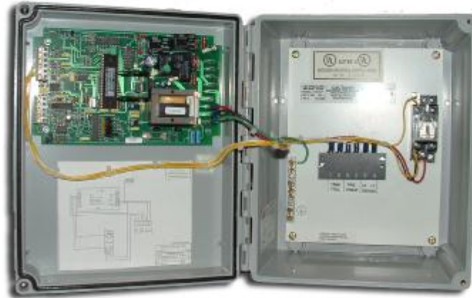
Fig. 3.4 Series 100 Inside Controller upgrade (Models 4040-1 to 4040-2)
