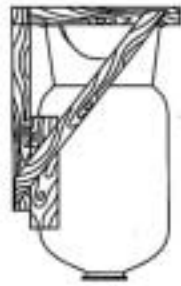
A pressure vessel with an integral Fiberglass base should be placed in a vertical upright position before removing its skid.
